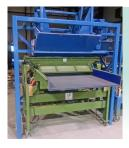
The RFM volumetric vibratory hopper feeder is a compact, self-contained unit featuring a bulk supply hopper with a vibratory feeder.
